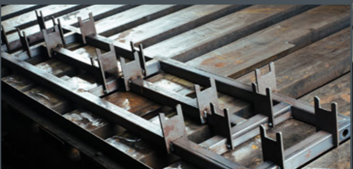
PRECISE, REPEATABLE PRODUCTION - WELDING JIG
